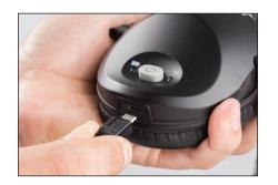
2 3 • **LED Indicators**—During operation, battery indicator ( ) begins blinking when there are approximately 3 hours remaining. While charging, battery indicator LED displays solid light and is off when fully charged.
